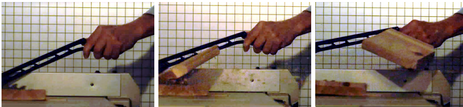
Figure 24: Kickback during cross-cut experiment at different time frames starting from the left-most image.
