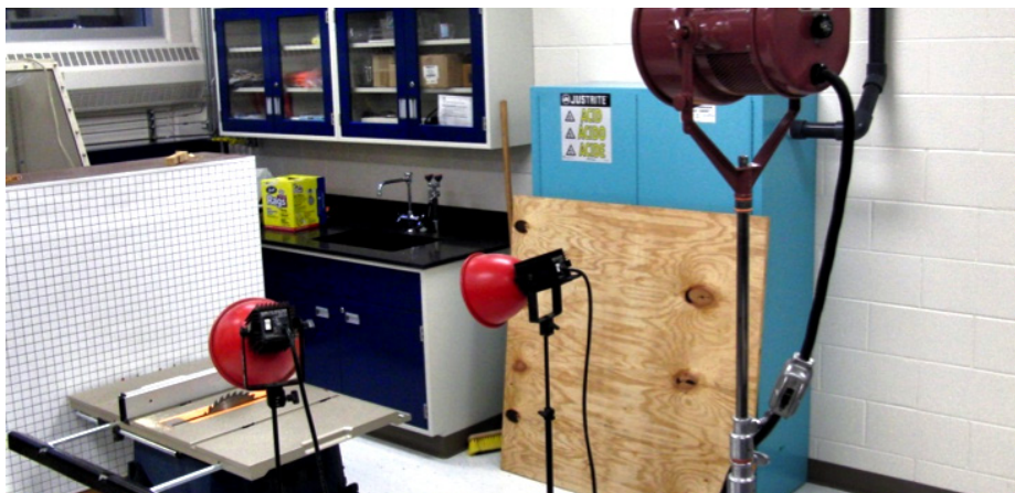
Figure 22: Experimental setup for kickback simulations
