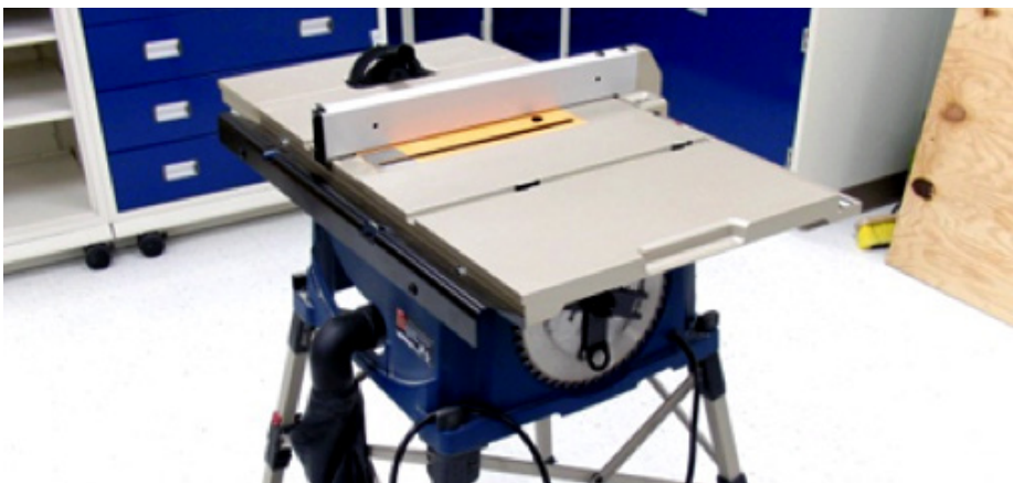
Figure 17: Photograph of direct-drive table saw used in experiments
