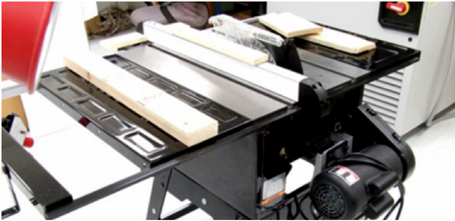
Figure 17: Photograph of direct-drive table saw used in experiments
