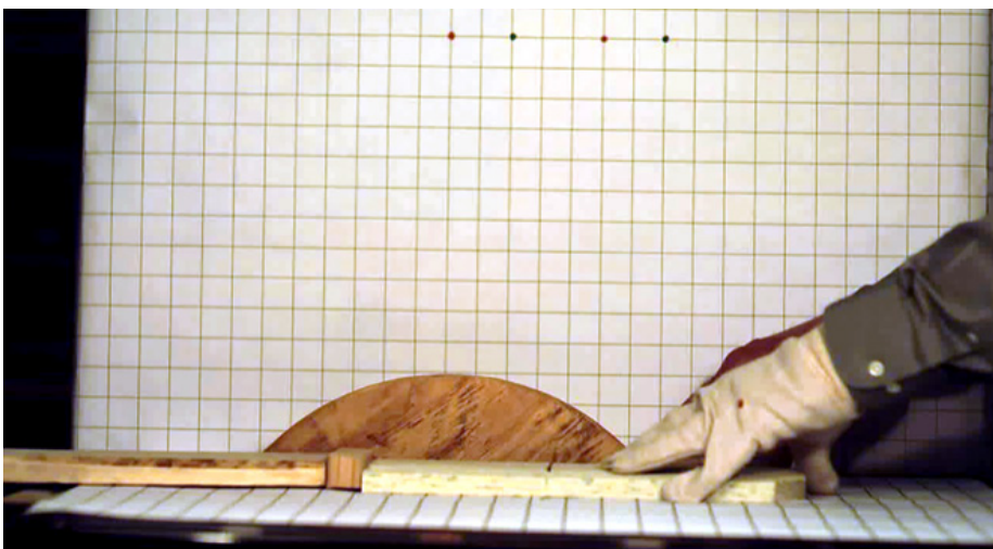
Figure 21: Reach-over test with falling board (left-most piece)
