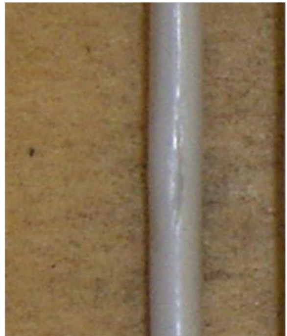
Figure 34 - NM Cable insulation cracked by 7ft-lb hammer impact
