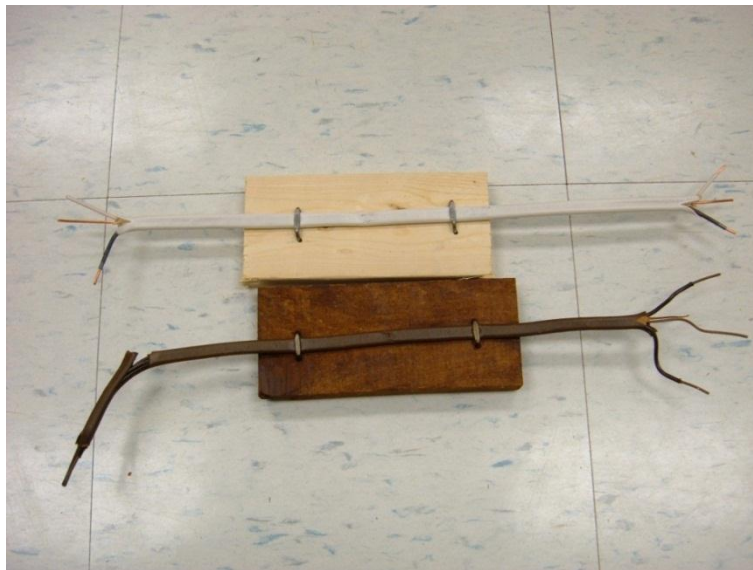
Figure 45 – Hammer-damaged and aged NM cable samples for the UL1449 test.
