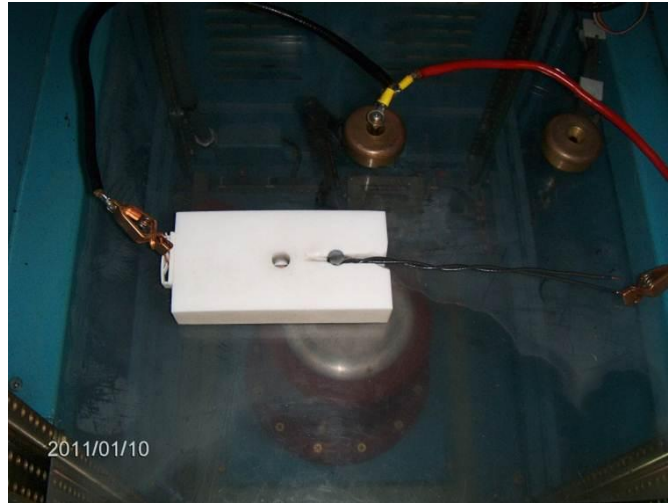
Figure 11 - Fixture for the NM cable breakdown voltage test
