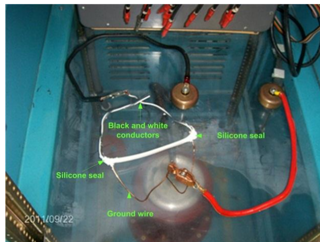
Figure 42 – Setup for the breakdown voltage test for intact NM Cable
