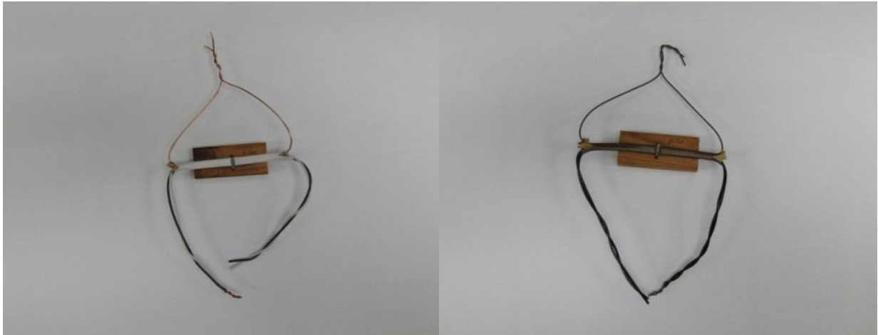
Figure 43 - Over-compressed NM cable B sample for breakdown test
