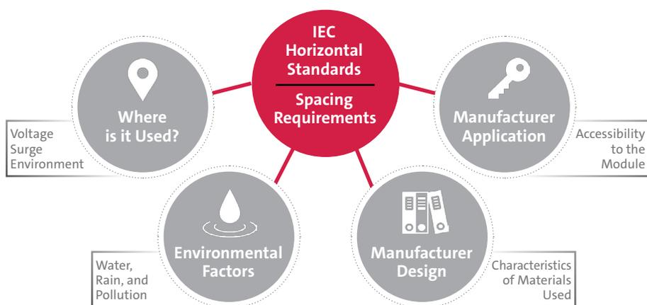
Construction requirements in UL 61730-1 are specific to PV module materials, equipment application, accessibility and environmental factors; when applied correctly they reduce the likelihood of technical error in the design stage. Applying the concepts of insulation coordination and getting the spacing's right increases confidence of a compliant result when testing for safety certification, reducing the cost of rework.
