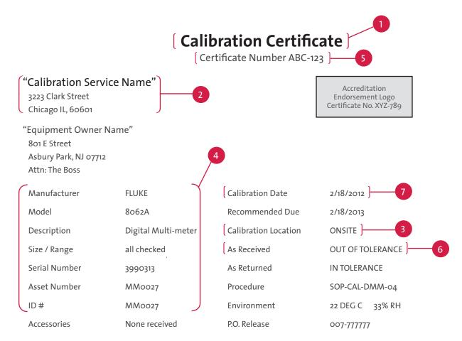
This instrument has been processed and calibrated in accordance with "Calibration Service Name" Quality Assurance Manual and is traceable to the National Institute of Standards and Technology (NIST). The "Calibration Service Name" quality system is registered to ISO 9001:2008, A2LA - accredited to ISO / IEC 17025 – 2005 & ANSI /NCSL Z540-1-1994, and compliant with ISO 10012-1, 10 CFR 50 App. B, 10 CFR 21, NQA-1 and MIL-STD-45662A. This report may not be
